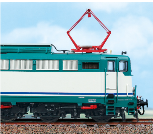
Locomotiva E646 101 navetta in livrea XMPR con griglie bianche. OML Roma San Lorenzo. Electric locomotive E.646.101 for push-pull trains in XMPR livery. Roma S. Lorenzo Depot. E-Lok E.646.101, in XMPR Lackierung für Pendelzüge. Bw Roma San Lorenzo.
