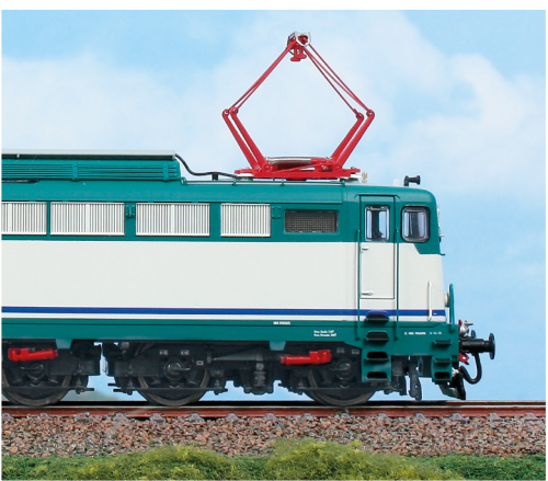
Locomotiva E646 127 navetta in livrea XMPR con logo frontale di Tipo 3. IMR Firenze. Electric locomotive E.646.127 for push-pull trains in XMPR livery. Firenze Depot. E-Lok E.646.127, in XMPR Lackierung für Pendelzüge. Bw Firenze.
